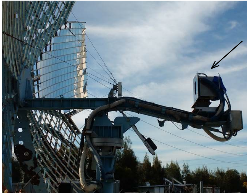
Figure 2 – The receiver/storage unit (arrowed) mounted on the parabolic dish.
